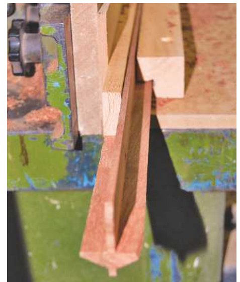
▲ Pic.14 The supports to stop the break-out during moulding the glazing bars
